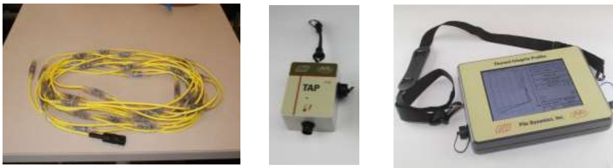
Figure 15 Thermal Integrity Profiling Assembly with TIP wires, TAP and Readout Unit
